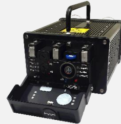
Ground Based Data Transfer Unit
